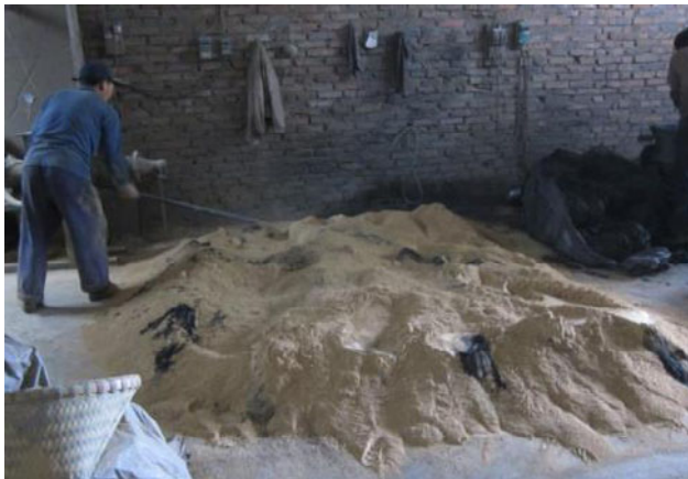
Figure 6. Yingjing grinding room, where milled clay and selected, ground coal cinders are mixed together and then wetted and pugmilled before use in the potting rooms.
