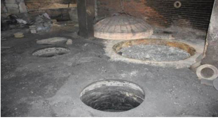
Figure 21. Primary firing kiln filled with coal cinders has dome cover behind; two glaze kilns at back left; in the foreground is the glaze kiln for teaware and the teaware kiln is off image at right.
