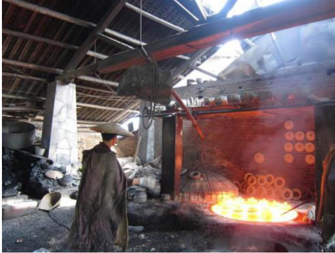
Figure 23. The kiln cover is levered off when pots are orange-hot. Note pots and lids above and behind the kiln, as well as setter rings, are preheating. These objects will be fired next.
