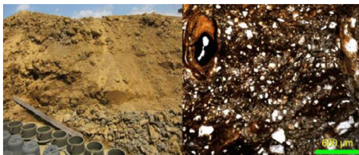
Figure 4. Yellow clay (left) purchased from farmers is rich in illite, quartz, and organic material, along with iron oxides and accessory chlorite mica; right shows a thin section of the yellow clay in plane polarized light.
