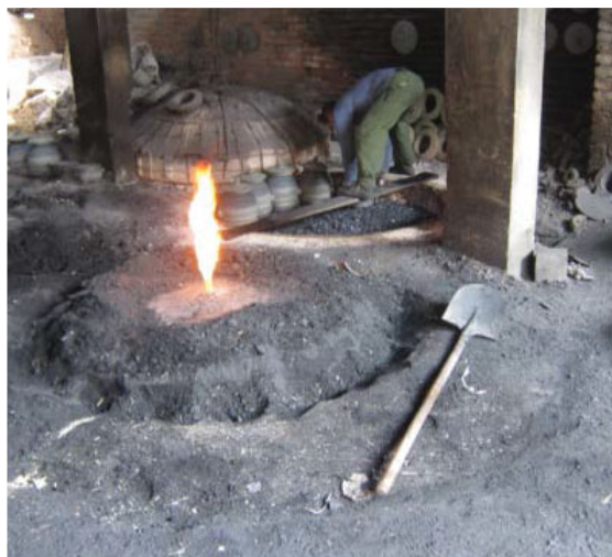
Figure 26. A reduction fire releases flames and smoke when the metal lid is placed on the glaze kiln. The worker then immediately begins to prepare the primary kiln bed for the next firing.
