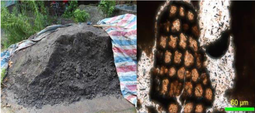
Figure 7. Black Gaoxian illitic clay (left) is filled with iron oxides and carbonized organic material; some of the organic structures are filled with secondary calcium carbonate (right) as shown in this thin section in plane polarized light that has been stained for calcium carbonate.
