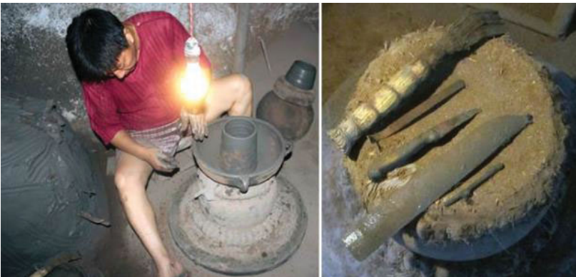
Figure 12. Gaoxian master potter, Huang Bin Xue, builds a brazier or “Sichuan hotpot” on a low kick wheel (left). The clay body supply is to the left and water is to the right. His hand-made tools (right) are kept near the workstation (a large brush to add and spread water, hook to shape joints, knife, trimming tool, and needle tool).
