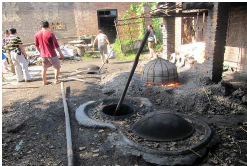
Figure 28. In Gaoxian a shallow ash-glaze pit with metal lid (no fuel, only leaves) is located in front of the primary pit (coal-fired to about 1050°C). The long, hooked rod for transferring pots is in the glaze kiln. A second pit and lid are in the background on the other side of the firing pit.
