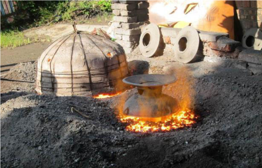
Figure 27. In Gaoxian, two pits are dug in a coal bed, one for pre-heating a single pot, the other for firing an already-heated pot under a small removable dome of similar design as in Yingjing.
