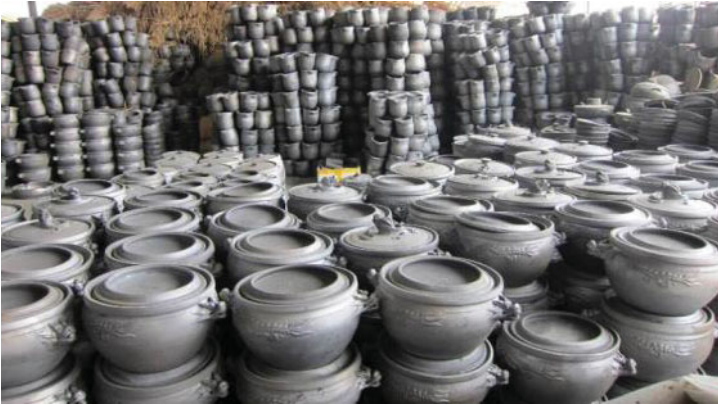
Figure 1. Coal-clay ceramics with an ash glaze are black with a silvery, bubbly surface texture.
