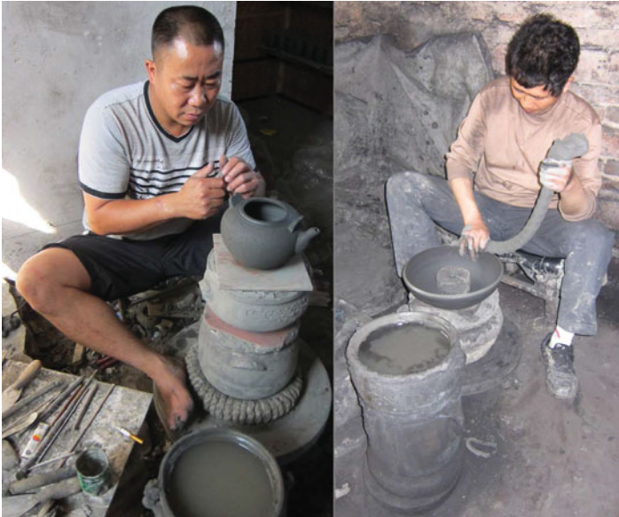
Figure 10. Master potter Zeng Qinghong (left), assembles a teapot above a kickwheel on a raised working surface; another potter (right) is adding coils to a mold-formed base made the previous day. He has chosen a lower-height working surface on which he will add two coils, then paddle and throw each, to build the walls and form the rim of a rice pot, one of 50 or 60 he will complete this day, and similar to the one with floral decoration below the teapot (left).
