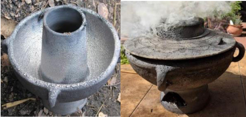
Figure 36. A brazier, the most typical product of the Gaoxian workshop, has an interior silvery, bubbly, and glassy texture from the ash glazing process (left); in cooking use (right) with coals on the grate and ash collecting in the base. Different foods can be cooked quickly in succession to change and add to the flavor, and kept hot on the table during the course of a long banquet.
